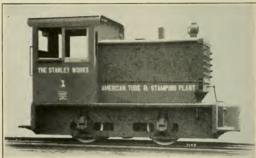
15-ton, 110 H.P. gasoline electric locomotive, used in steel mill work.
